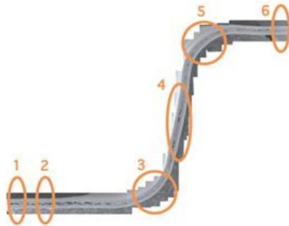
**Figure 4.** Measuring positions after cutting the drawing cups.
