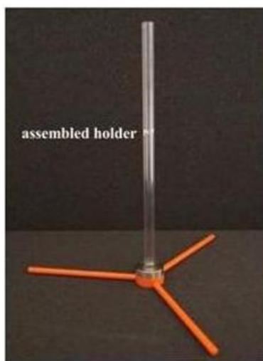
**Figure 5.** Assembling the IAEA standard holder for the RPLD irradiations.
