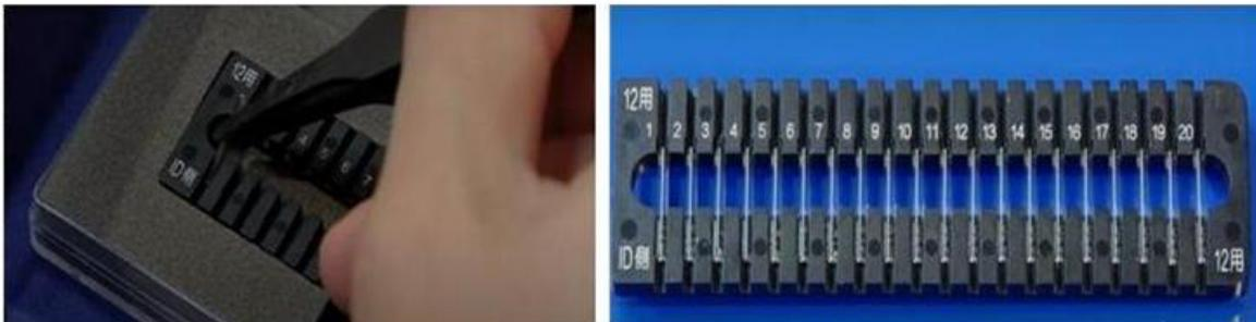
**Figure 4.** FGD-1000 reader can read up to 20 glass rods.
