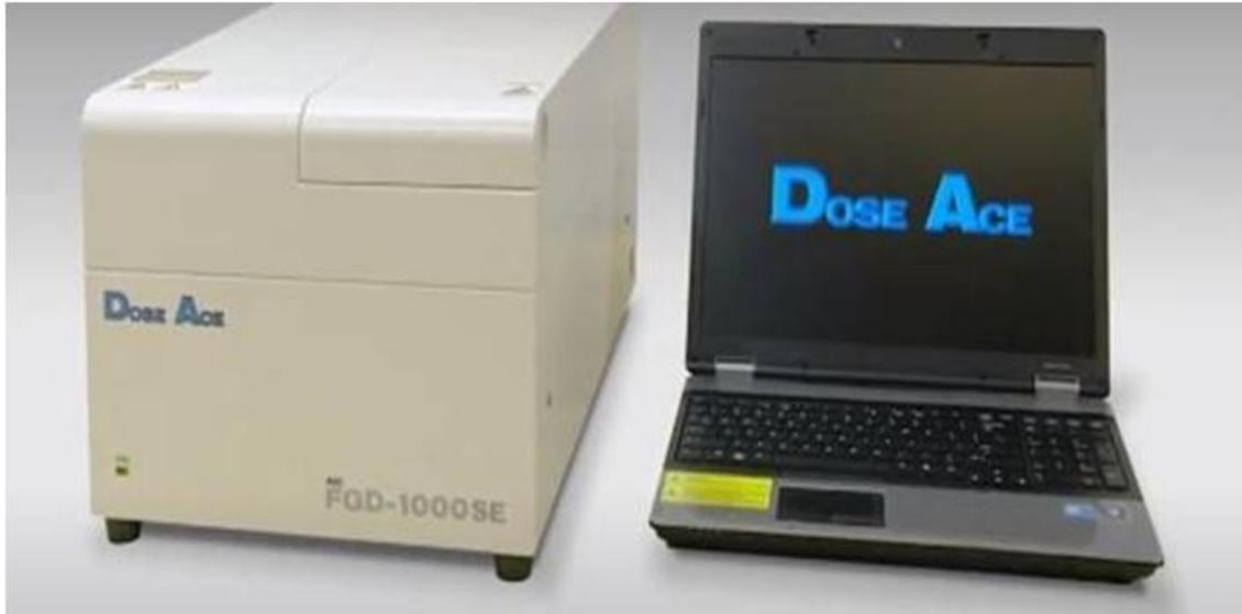
**Figure 1.** Dose Ace system consisting of GD-302M glass rods and a FDG-1000 reader from Asahi Techno Glass Corporation (ATG) is used in IAEA Dosimetry Laboratory.
