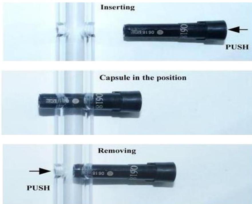
**Figure 7.** Different positions of the capsule with RPLD – Inserting, Capsule in the position and Removing.
