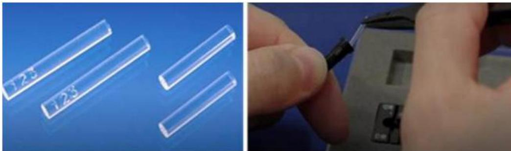
**Figure 2.** The glass rods- in the left and watertight capsules - in the right.
