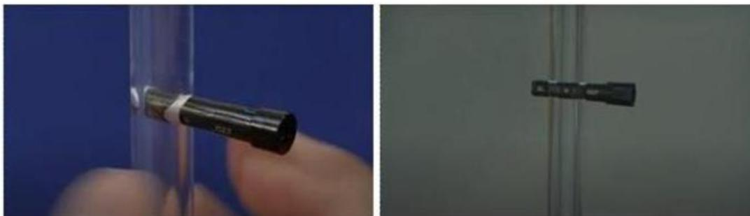
**Figure 3.** ID number and bar code of the capsules - in the left. The sensitive area is marked on the capsule - in the right.
