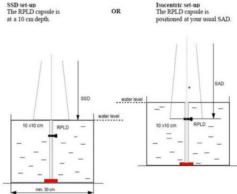
**Figure 6.** Two alternative geometry set-ups for the RPLD irradiation.
