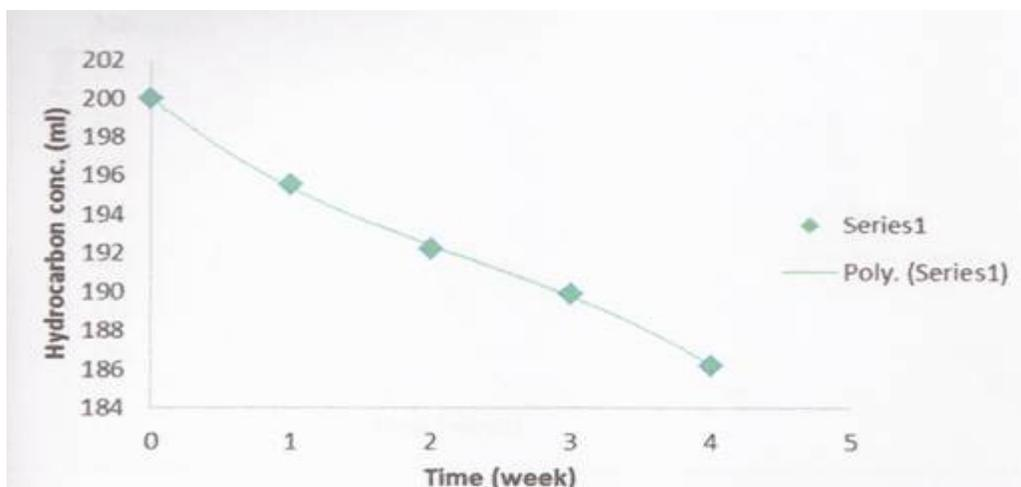
Figure 8. Graph of hydrocarbon conc. against time for sample B
