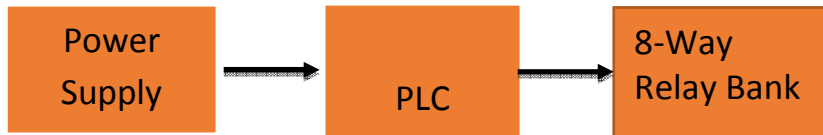
Figure 3. Block diagram of the PTS control unit
