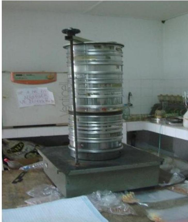
**Photo 4.** Granulometer consisting of several sieves with diameters between 5.00 and 0.315 millimeter.
